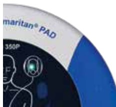
Figure 10. Flashing green LED; no action required.
